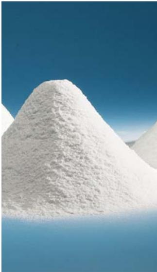
3M™ Glass Microspheres can reduce the weight of plastisols, used for underbody coating and seam sealer, by up to 50% – contributing to lower overall vehicle weight, and helping to meet increasingly-stringent CAFE standards. At the same time, 3M glass microsphere-filled plastisols can reduce costs by 15–20% over conventional plastisol fillers, in many applications.
